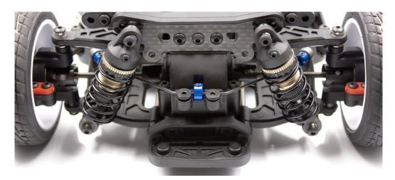
(Pictured: Shock and anti-roll bar sets installed on the Apex2.)
