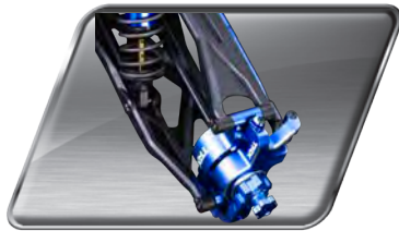
Aluminum C-hubs and Steering Blocks
