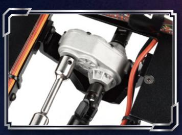
The Trail Finder 2 Chassis includes the Hammer Transfer Case that features a cast metal exterior and heavy-duty .8 Mod Widened Gears, ensuring lasting functionality.
