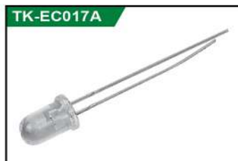
TK-EC017A 5mm LED (白灯发红光) 5mm LED (white LED shine red light)
