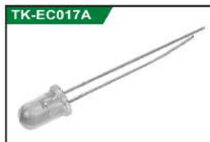
05mm LED (白灯发红光) 05mm LED (White LED shine red light)
