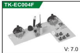
7.0发射板(2.4GHz) 7.0 Transmitting board (2.4GHz)
