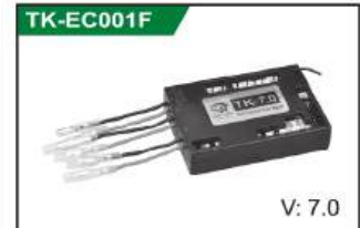
7.0功能主板(2.4GHz) 7.0 Multi-function circuit unit (2.4GHz)
