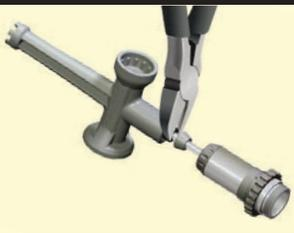
C. Remove/Install Rod End
