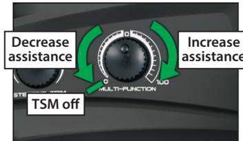
When driving on surfaces with some traction, decrease the TSM setting to allow the vehicle to feel more "loose" for power sliding, drifting, and so on. On surfaces with very little traction (loose dirt, smooth concrete, ice/snow), increase TSM to maximize acceleration and control.
