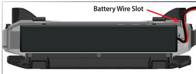
3. Make sure the battery is snug in the compartment. Use the included springs and/or retainers, if necessary.
