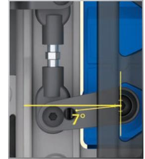
If necessary, fine-tune the length of the second steering link to eliminate any load on the steering system in the neutral position. If you are using aftermarket servos, it is important to use servo horns designed for E-Revo. Optional steering servo horns are sold separately for use with non-Traxxas servos.
