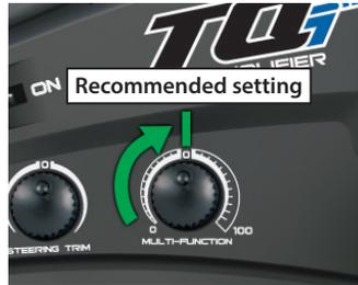
Turn the knob clockwise to increase assistance; turn the knob counterclockwise to decrease assistance. Turn the knob counterclockwise to its stop to turn TSM completely off. **Note:** TSM is deactivated automatically when driving or braking in reverse.
