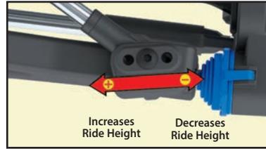
The ride height can be finely tuned by adjusting the sag of the suspension. **Do not attempt to make large changes to the ride height by adjusting the spring pre-load on the shock bodies.** If suspension sag is severe and requires a large increase of the spring pre-load to compensate, then a firmer spring should be used.
