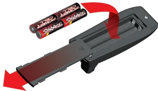
2. Install the batteries in the correct orientation as indicated in the battery compartment.
